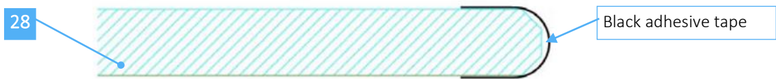
Fig. 24 Application of black insulation tape along the edge of the small mirror
