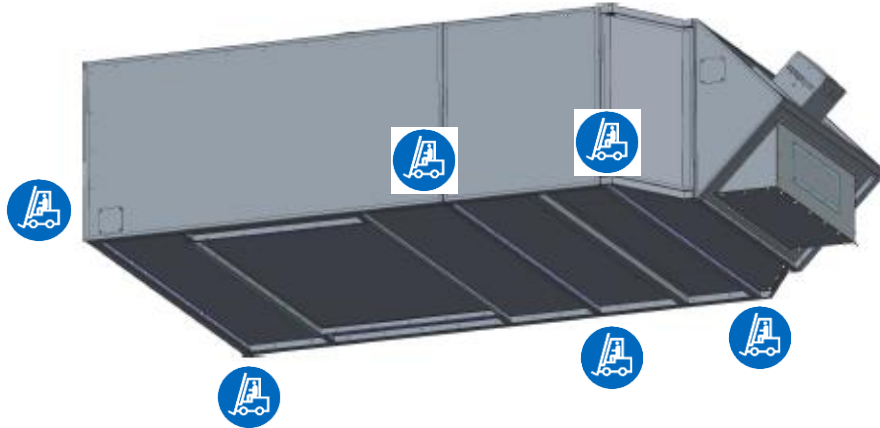
Fig. 51 Lifting points for CoeLux® 45 HC
