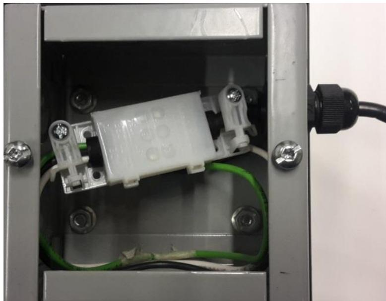
Fig. 40 Completed electrical connections to the projector 74-00013-01
