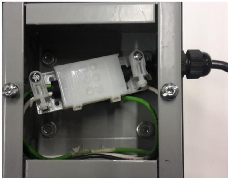
Fig. 38 Completed electrical connections to the projector 74-00013-01
