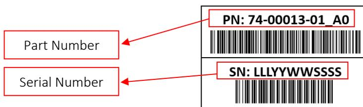
Fig. 2 Label with Part Number and Serial Number
