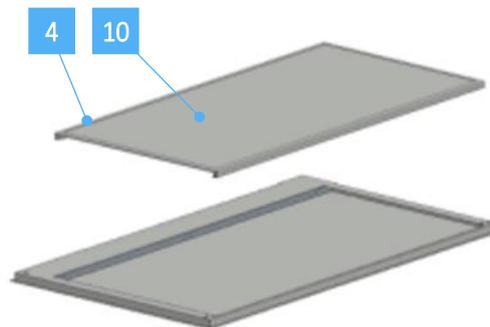
Fig. 21 *Inserting the mirror frame in the lid*
