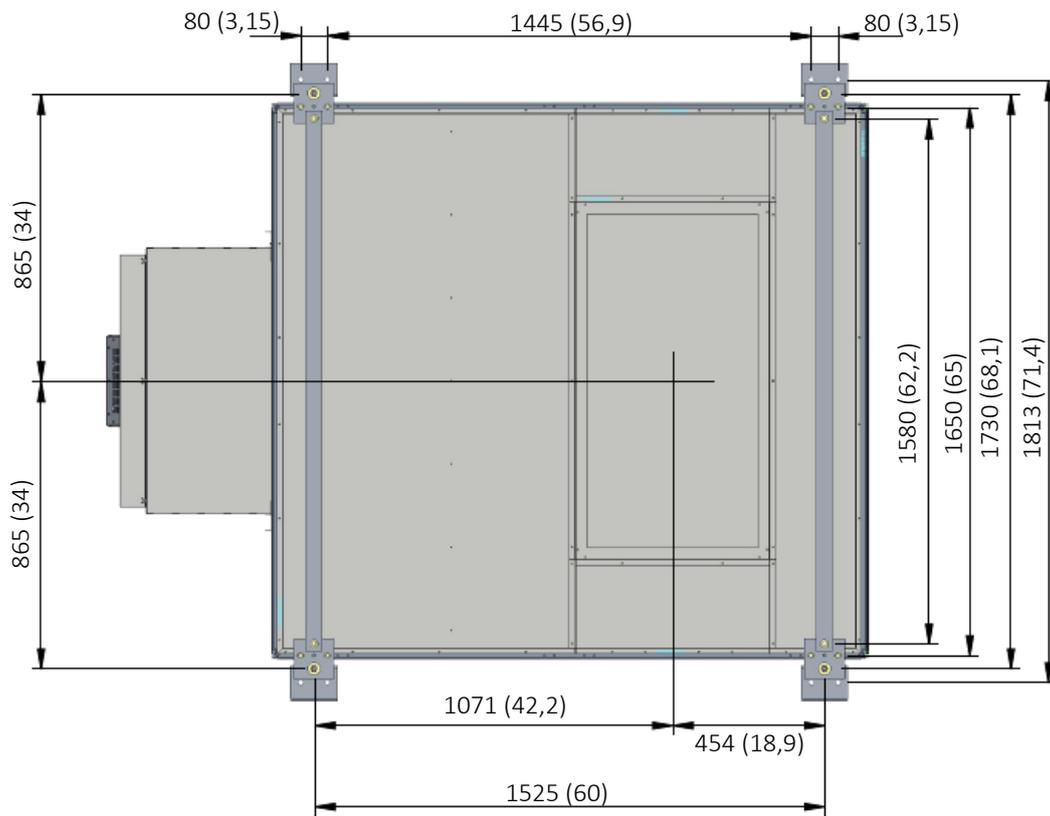
Fig. 54 Suggested anchoring system – Bottom view
