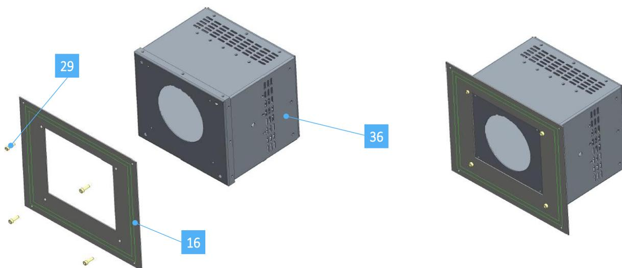
Fig. 29 *Securing the projector on the plate*
