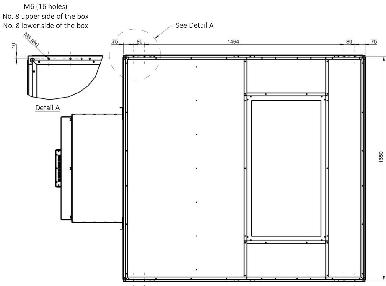
Fig. 47 Profile or plate fastening holes
