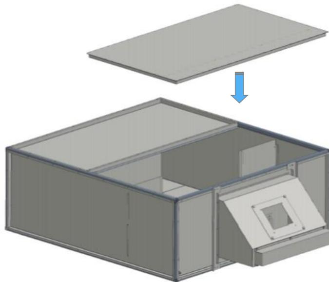
Fig. 23 *Inserting the upper lid on the box*
