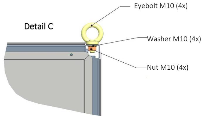
Fig. 58 Recommended anchoring system – Option 2
