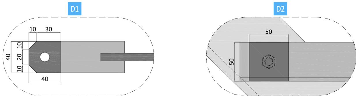
Fig. 61 Details D1 e D2: inserts for hanging system angled dark-box
