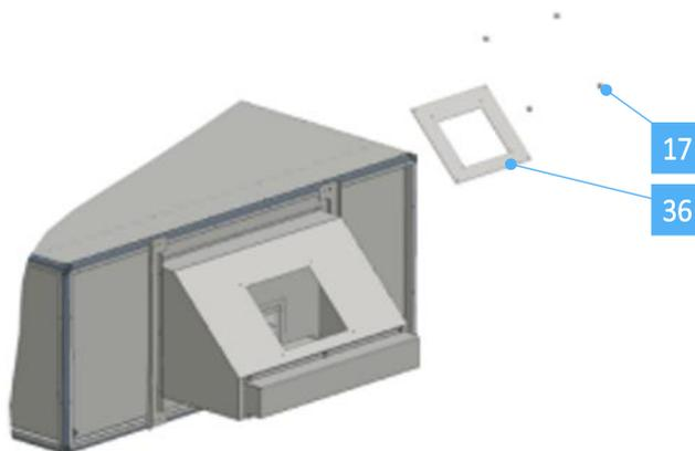
Fig. 28 *Plate removal*
