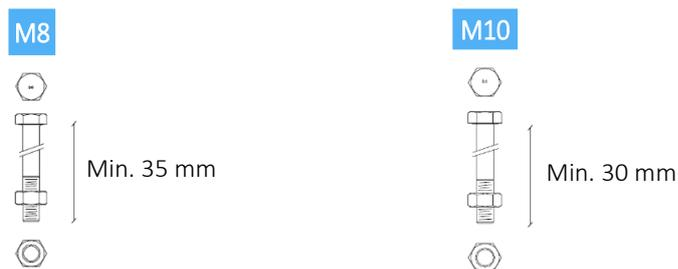
Fig. 64 Bolts M8 and M10
