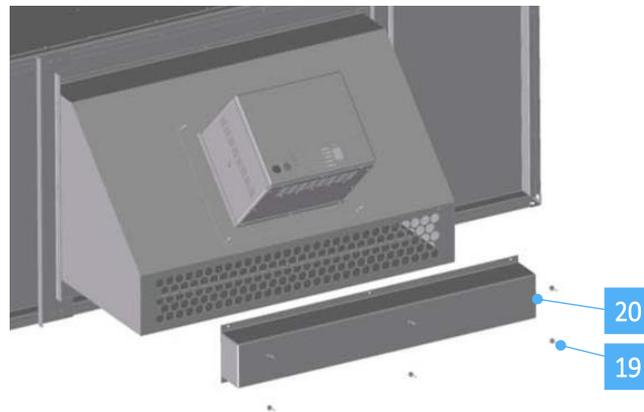
Fig. 44 *Silica-gel box removal*
