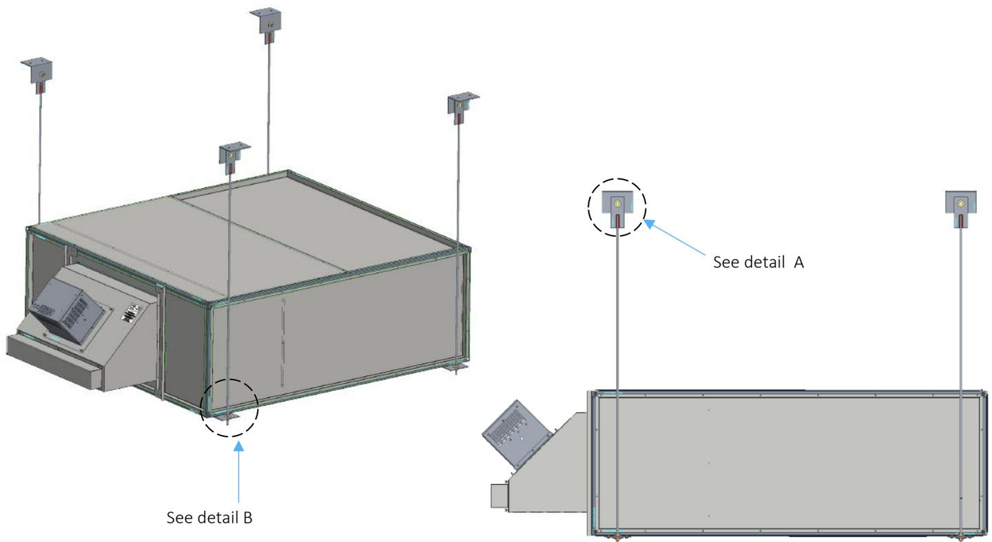
Fig. 53 Suggested anchoring system
