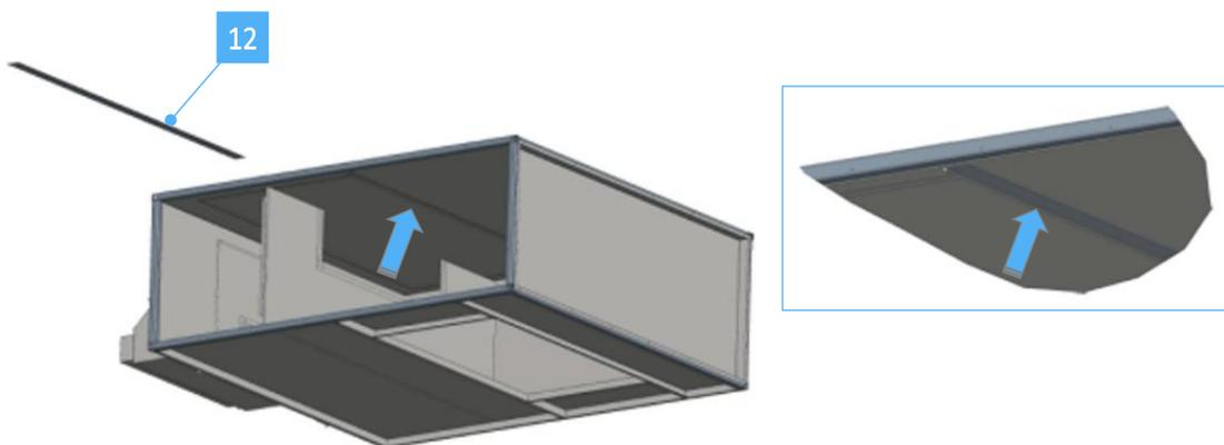
Fig. 24 *Positioning the magnetic strip*
