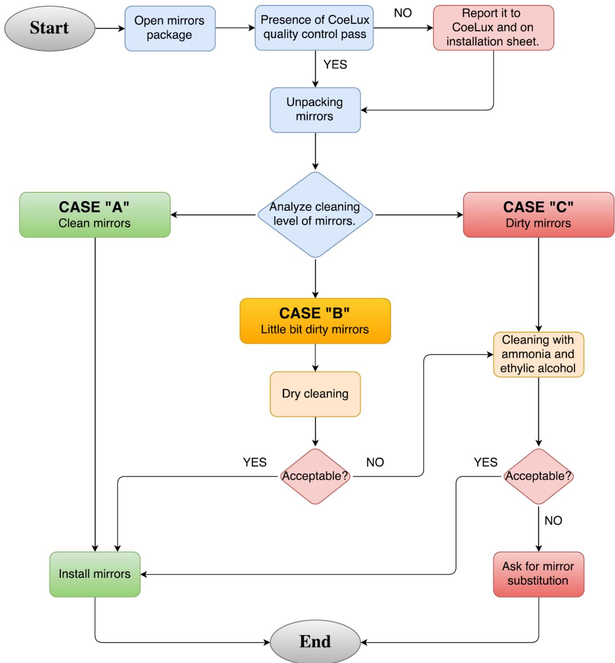
Fig. 3 Flow chart analysis and extraordinary cleaning procedure of mirrors
