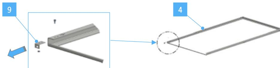
Fig. 18 *Bracket removal*
