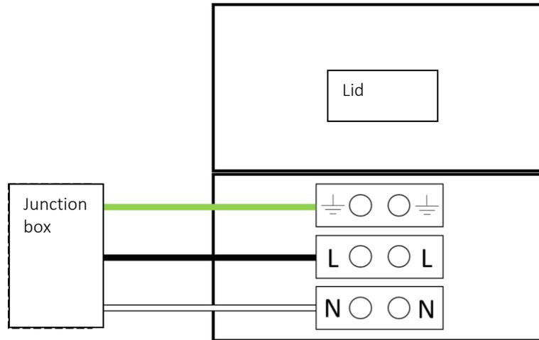
Fig. 37 Sketch to show an example of the terminal board supplied
