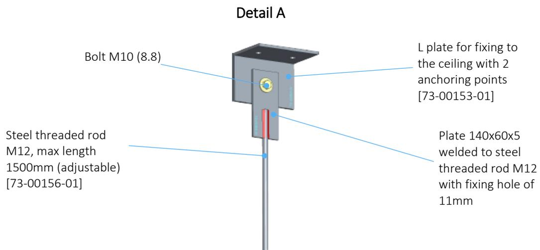
Fig. 55 Suggested anchoring system – Detail A
