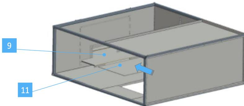
Fig. 11 *Inserting the small mirror*
