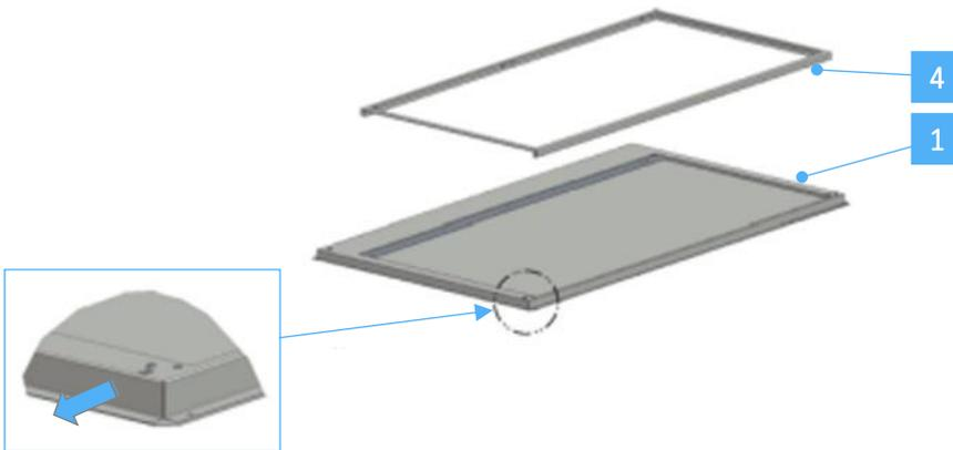
Fig. 16 *Frame removal*
