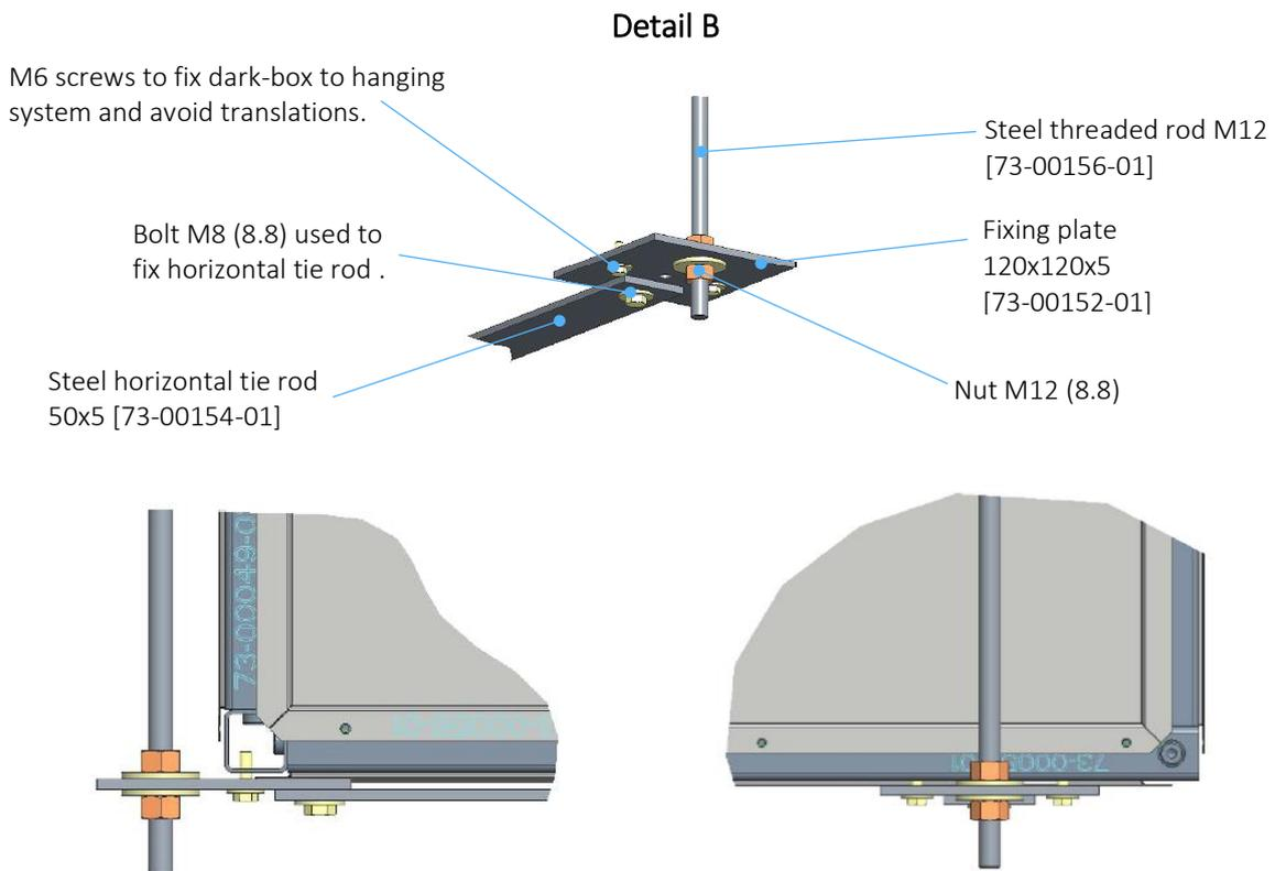
Fig. 56 *Suggested anchoring system – Detail B*
