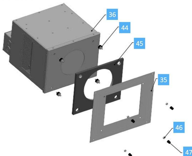
Fig. 31 Installation of the ventilation kit
