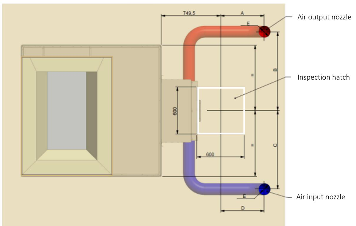
Fig. 50 *Inspection hatch and ventilation nozzle layout*
