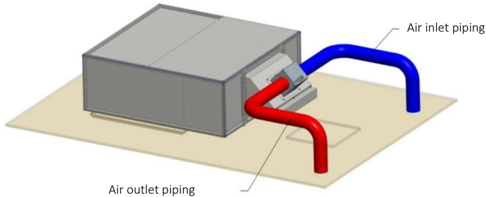
Fig. 51 Ventilation nozzle connection diagram
