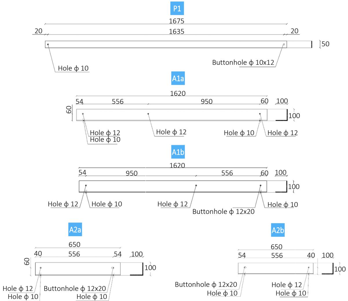
Fig. 63 Components P1, A1a, A1b, A2a e A2b
